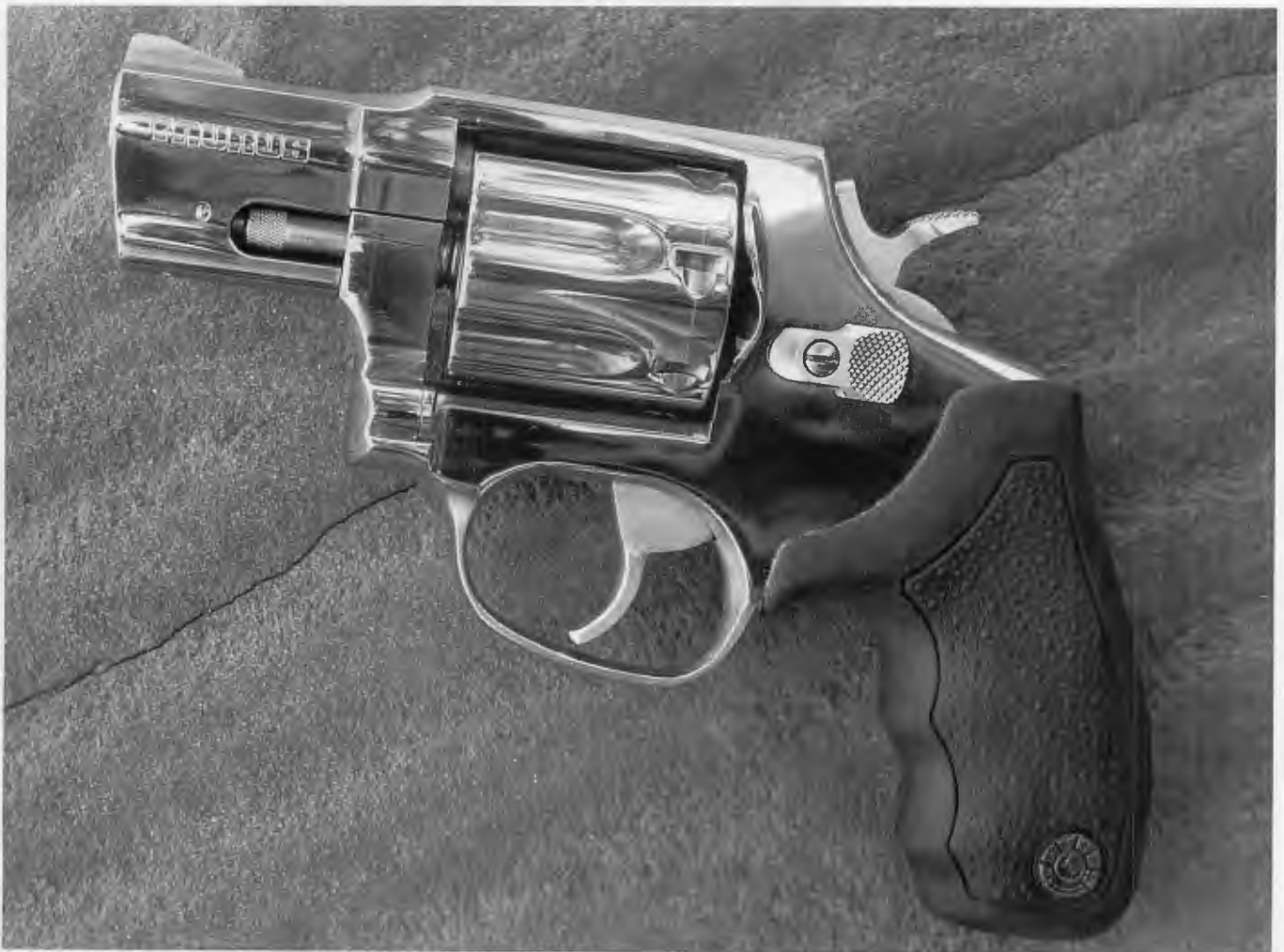
Seven beans in the wheel; Taurus M617 revolver provides as much fire-power as an original M1911 seven-round magazine. (below) Taurus M617 .357 Magnum snubnose, left-side view. Note integral full-length barrel shroud and cylinder latch, which is patterned after that of Smith & Wesson and must be pushed forward to swing out the cylinder.
